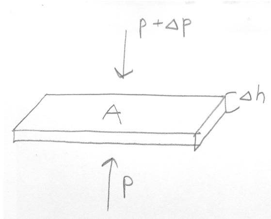
Figure 1: pressure balanced
