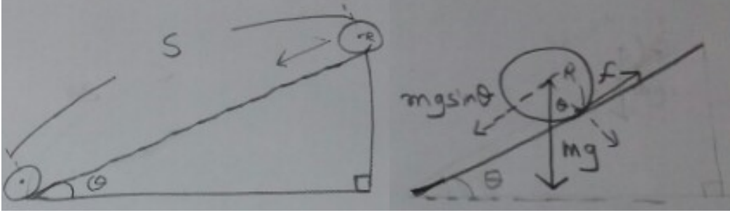
Figure 1: Rolling down on an inclined plane
